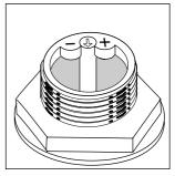
necessary, rotate the ring in the anticlockwise direction from the "\_" setting towards the "+" sign, based on the hard-ness of the water being used.
